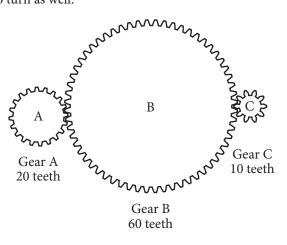
If Gear A is rotated by the motor at a rate of 100 rpm, what is the number of revolutions per minute for Gear C?
